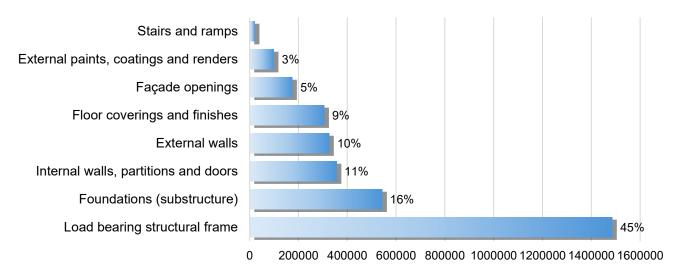
Figure 31 Structural Elements wise % distribution of total Embodied Carbon, School – MP
