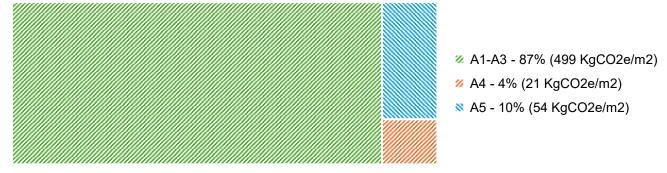
Figure 6: Distribution of Embodied Carbon in A1 to A5 Life cycle stages, Admin Building, Bengaluru
