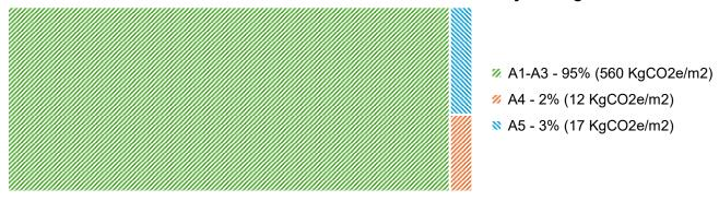
Figure 39 Distribution of Embodied Carbon in A1 to A5 Life cycle stages
