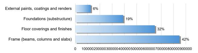
Figure 16 Structural Elements wise % distribution of total Embodied Carbon, International School.
