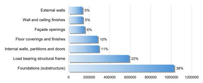
Figure 37 Structural Elements wise % distribution of total Embodied Carbon (EMC) office building
