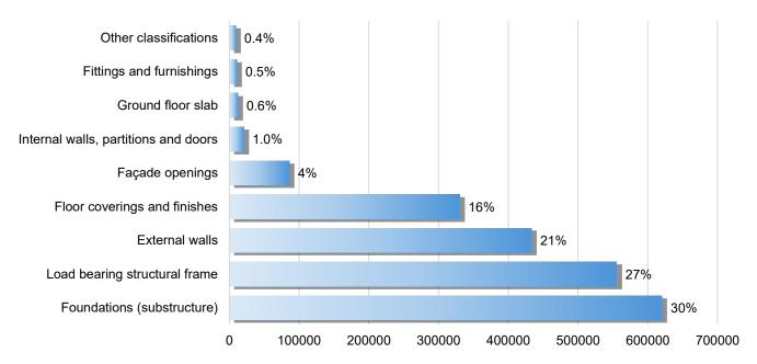
Figure 7 Structural Elements wise % distribution of total Embodied Carbon, Admin Building, Bengaluru
