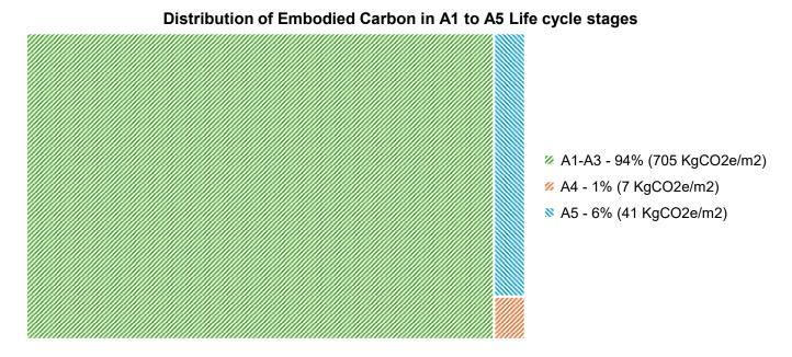
Figure 21 Distribution of Embodied Carbon in A1 to A5 Life cycle stages, Chandigarh Housing Board
