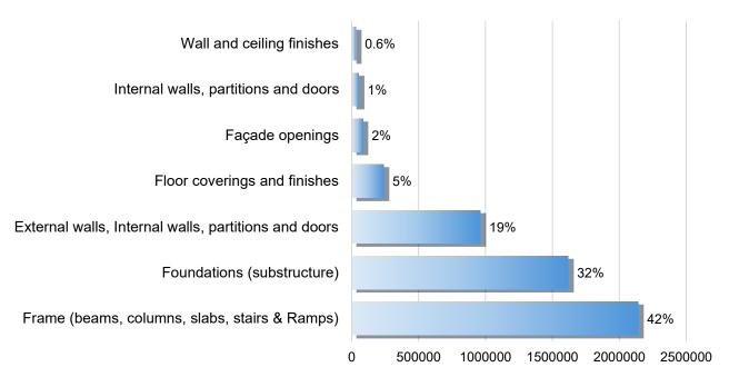
Figure 61 Structural Elements wise % distribution of total Embodied Carbon, Podar International School
