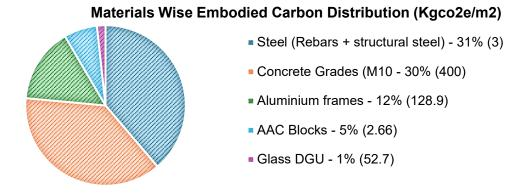
Figure 41 Materials Wise Embodied Carbon Distribution (Kgco2e/m2)
