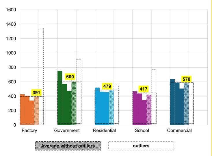
Figure 78 Embodied Carbon Benchmarking across typologies.
