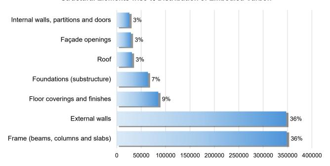
Figure 43 Structural Elements wise % distribution of total Embodied Carbon, Sawanand Apartments, Pune, Maharashtra
