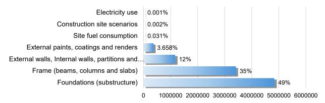
Figure 52 Structural Elements wise % distribution of total Embodied Carbon, Sri Govind Guru University – Admin Block
