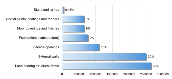
Figure 25 Structural Elements wise % distribution of total Embodied Carbon , Syal Architects Office
