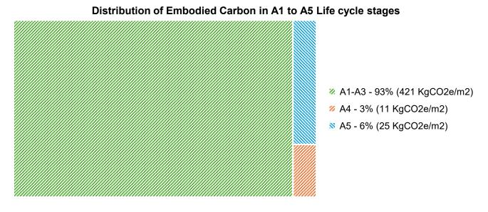
Figure 42 Distribution of Embodied Carbon in A1 to A5 Life cycle stages, Sawanand Apartments, Pune, Maharashtra
