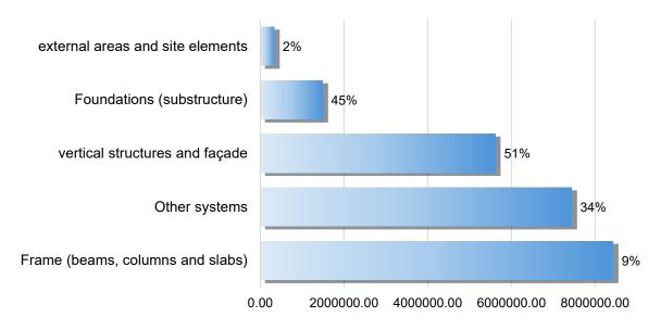
Figure 40 Structural Elements wise % distribution of total Embodied Carbon
