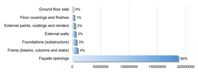
Figure 10 Structural Elements wise % distribution of total Embodied Carbon, Infosys Bengaluru
