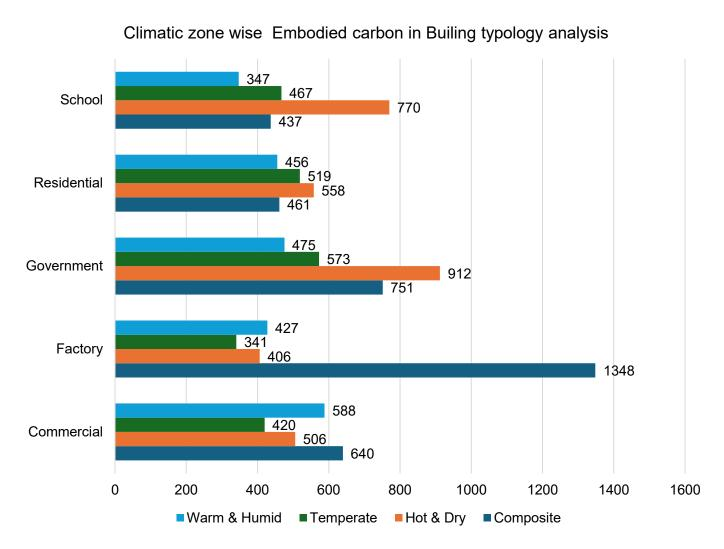
Figure 70 : Climatic zone wise Embodied carbon in Building typology analysis (KgCO<sub>2</sub> e /m²)
