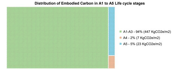
Figure 36 Distribution of Embodied Carbon in A1 to A5 Life cycle stages, (EMC) office building
