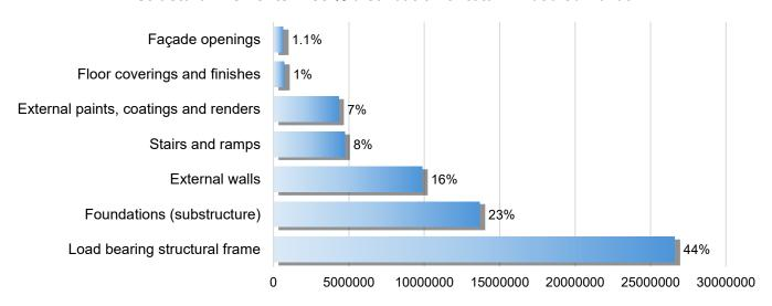
Figure 58 Structural Elements wise % distribution of total Embodied Carbon, Westin Residential.
