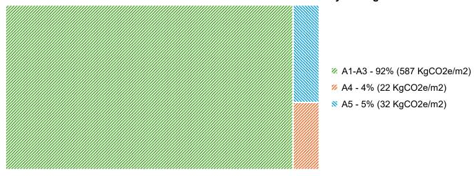
Figure 24 Distribution of Embodied Carbon in A1 to A5 Life cycle stages, Syal Architects Office
