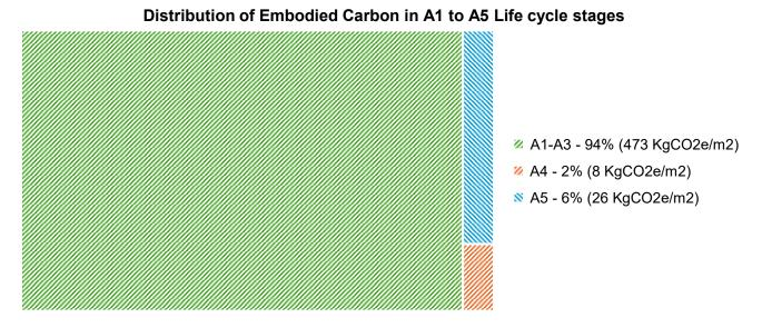
Figure 54 Distribution of Embodied Carbon in A1 to A5 Life cycle stages, Savvy Pragya.
