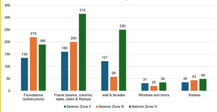
Figure 72 Structural element wise Embodied Carbon Footprint in Different Seismic Zones
