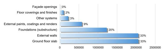
Figure 34 Structural Elements wise % distribution of total Embodied Carbon, Ramani Precision Machines, Mohali
