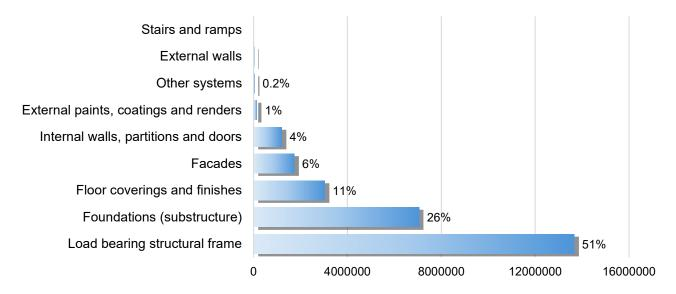
Figure 55 Structural Elements wise % distribution of total Embodied Carbon, Savvy Pragya.
