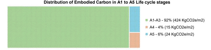
Figure 27 Distribution of Embodied Carbon in A1 to A5 Life cycle stages, Kanya Siksha Parisar
