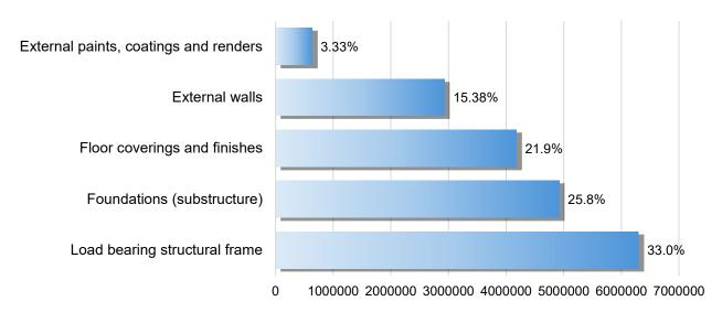
Figure 13 Structural Elements wise % distribution of total Embodied Carbon, Brigade Laguna
