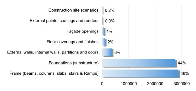
Figure 64 Structural Elements wise % distribution of total Embodied Carbon , Spirotech Factory
