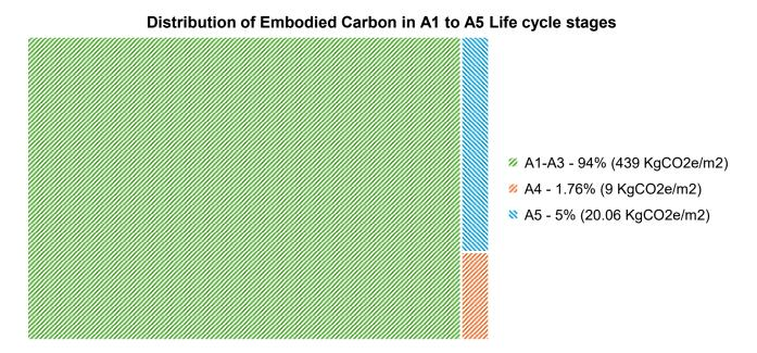
Figure 15 Distribution of Embodied Carbon in A1 to A5 Life cycle stages, International School.
