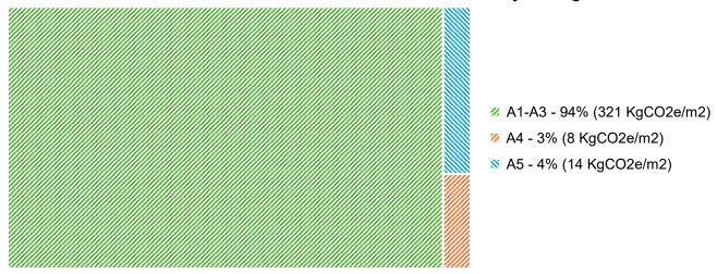
Figure 18 Distribution of Embodied Carbon in A1 to A5 Life cycle stages, Advik Factory (Bengaluru)
