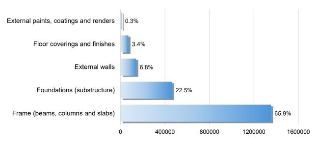
Figure 19 Structural Elements wise % distribution of total Embodied Carbon, Advik Factory (Bengaluru)
