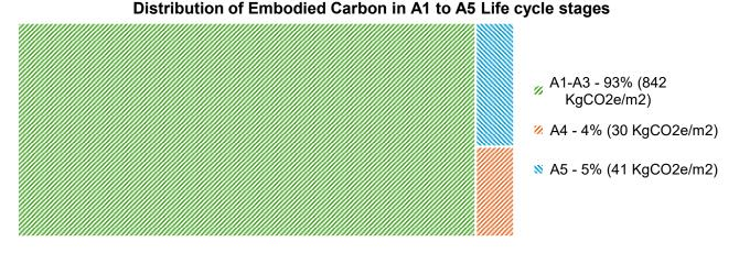
Figure 51 Distribution of Embodied Carbon in A1 to A5 Life cycle stages, Sri Govind Guru University – Admin Block
