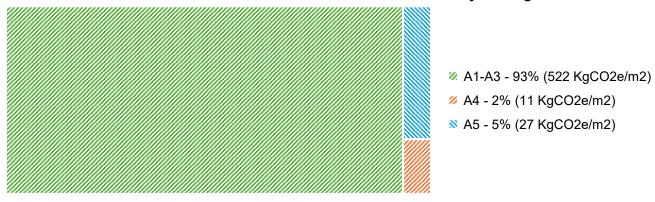
Figure 57 Distribution of Embodied Carbon in A1 to A5 Life cycle stages, Westin Residential
