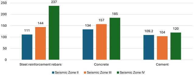
Figure 73 Material wise Embodied Carbon Footprint in different Seismic Zones
