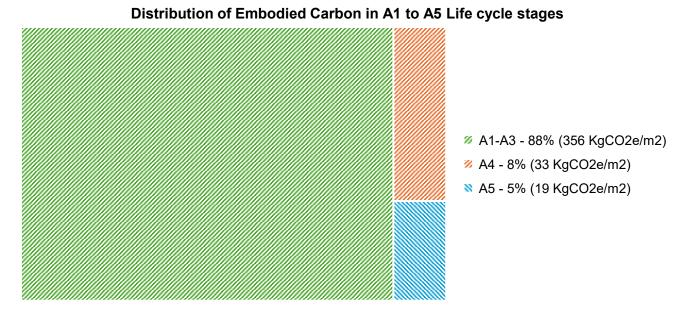
Figure 63 Distribution of Embodied Carbon in A1 to A5 Life cycle stages, Spirotech Factory
