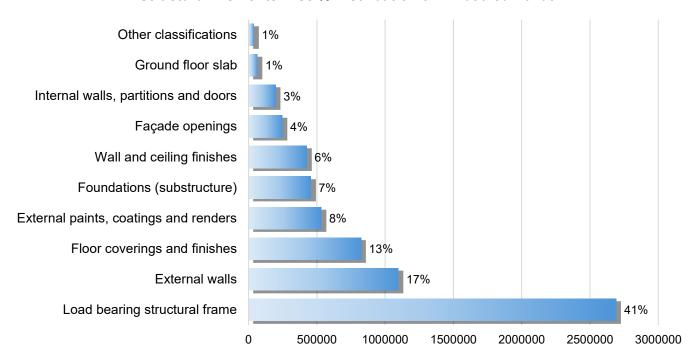
Figure 46 Structural Elements wise % distribution of total Embodied Carbon, PCMC Wakad School.
